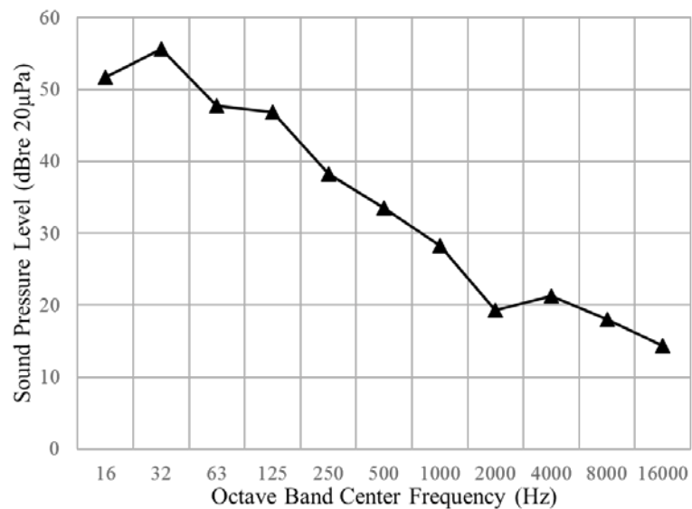
Figure 3.2 Measured octave band spectra for the ambient background noise in the test chamber when air-conditioning is off
